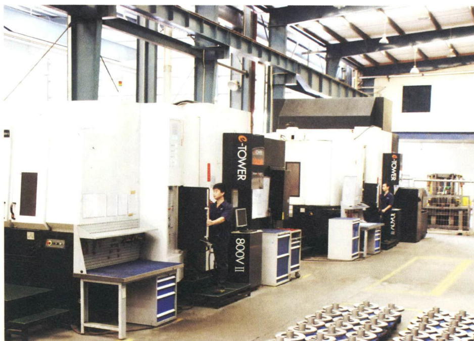
The 4-axis and 5-axis machine centre in the Tycon Shenzhen plant.
